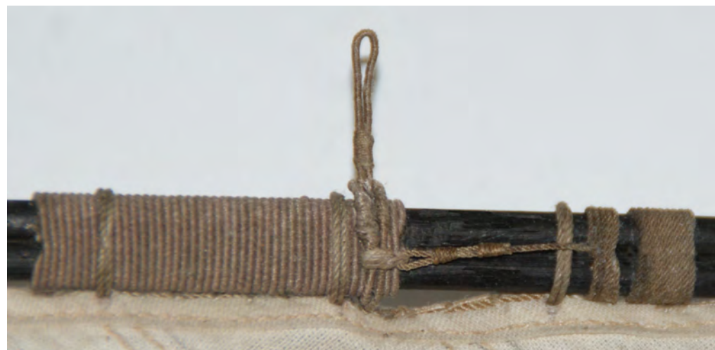
Photo n°. 226: The yard sling; at the side, the laniard/span. This laniard is a binding that keeps the sling from slipping.
