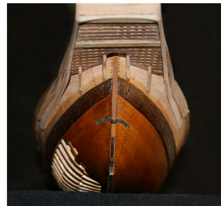
Photo n°. 123: A view of the underside. The small knees, support timbers for the wings, and cross-beam.
