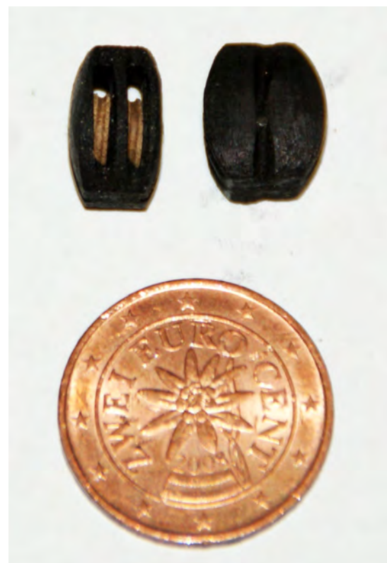
Photo n°. 207: Completed double blocks.
