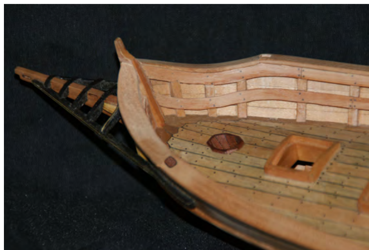
Photo n°. 107: Detail of the top rail at the stem. Note the two square openings for the bitts.
