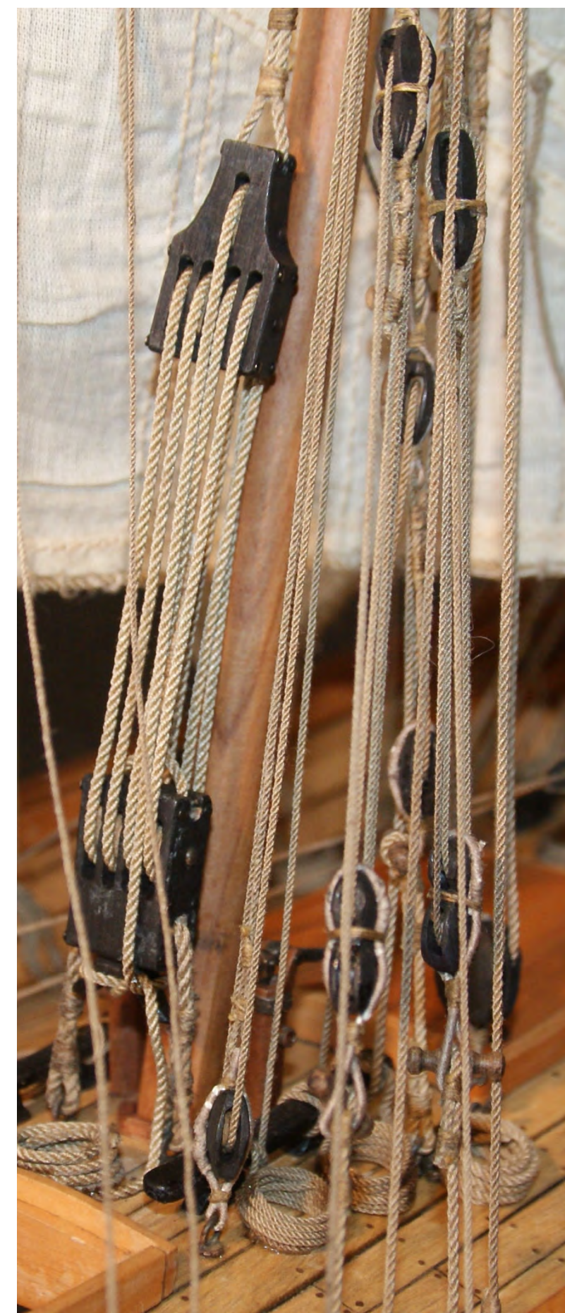
Photo n°. 230b: Detailed view of the upper large block. The fall of the tie reeves through the top of the large block, and is seized back to itself with three bindings.
