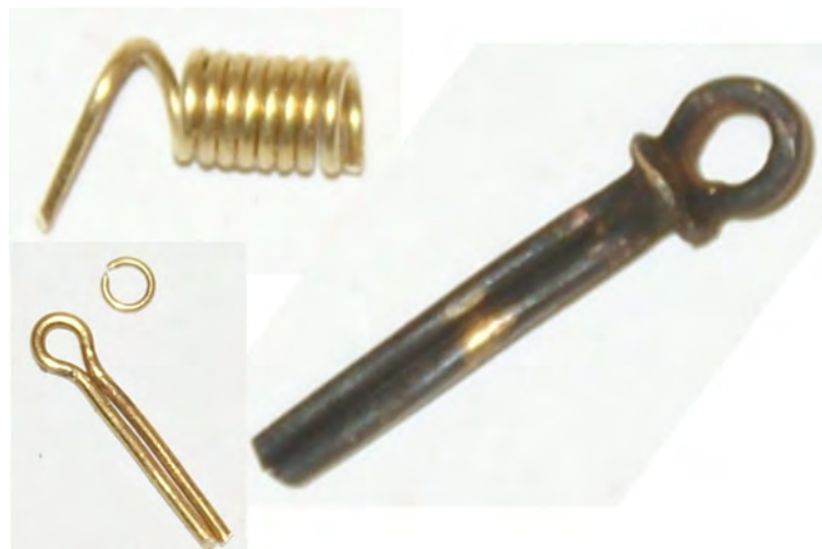
Photo n°. 179: The three elements and the completed and blackened eyebolt.
