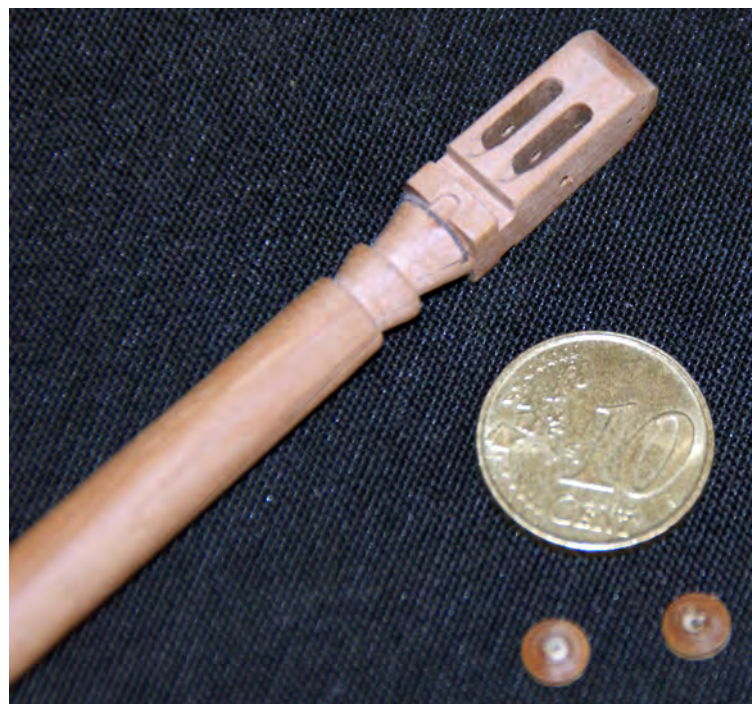
Photo n° 49: Detail of the « calcet » with the two sheaves.
