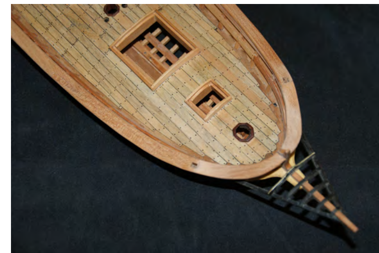
Photo n°. 104: Overhead view of the head with the top rail installed (61). Dimensions of the top rail: 1.5 x 8.
