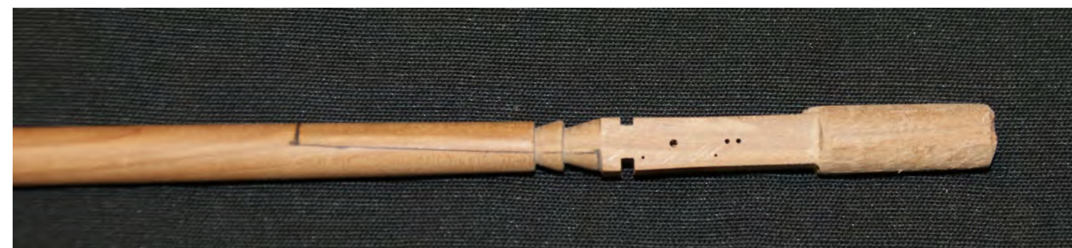
Photo n°. 46: The « calcet turned the other way shows the two slots, the hole for the sheave axle and two additional holes used in case of need. They are not rigged on this model.
