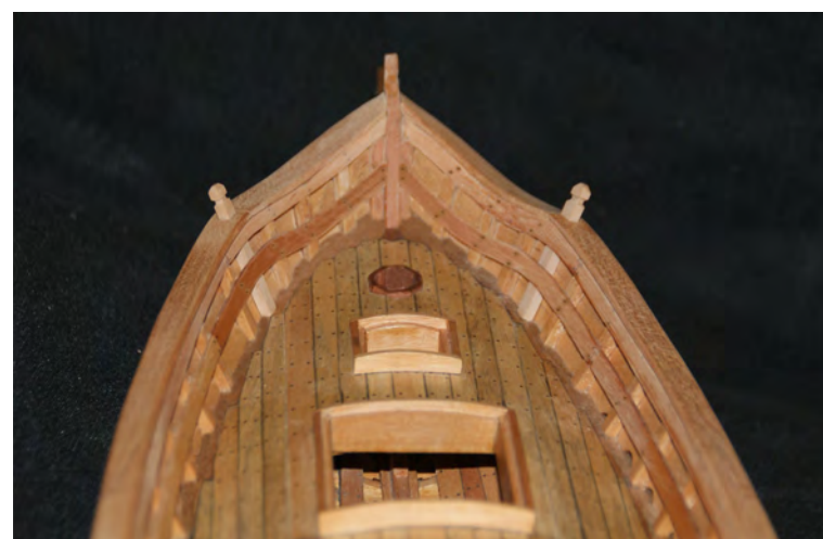
Photo n°. 110: The bitts are in place in the top rail. The foremast wedges (32), the small and main hatches are in place.
