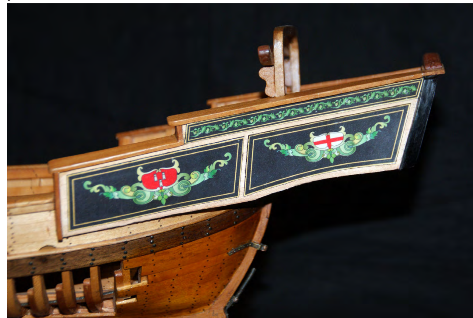
Photo n°. 140: Completed structure of the stern. The top of the rudder juts through the helm-port and the tiller is in place.
