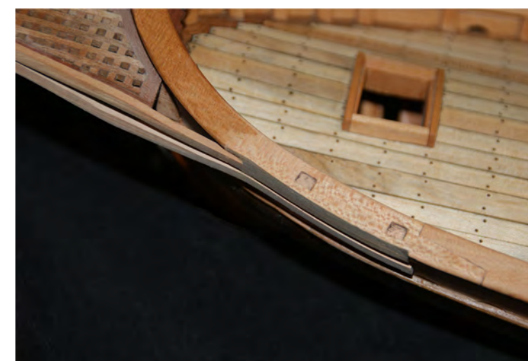
Photo n°. 121: A view of the side of the hull. The two rectangular holes are for vertical risers that; will serve to anchor the sides of the cadrega. Below the longitudinal timbers that support the wings.
