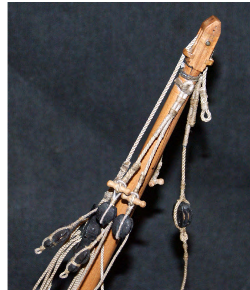
Photo n°. 222: Detail of the pendants - The masthead seizings are identical on both masts, only the size varies. Pendants 108 and 112 (main). The pendant (108) is served over half its length - this rope will need to be seized securely to the mast with very tight turns where it is folded back (see photo). Photo n°. 245:
