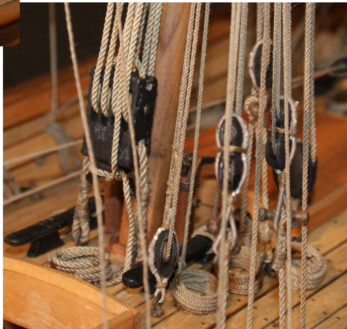
Photo n°. 259a: In the foreground, the lift of the lower half of the yard and at the top, the fiddle block.
