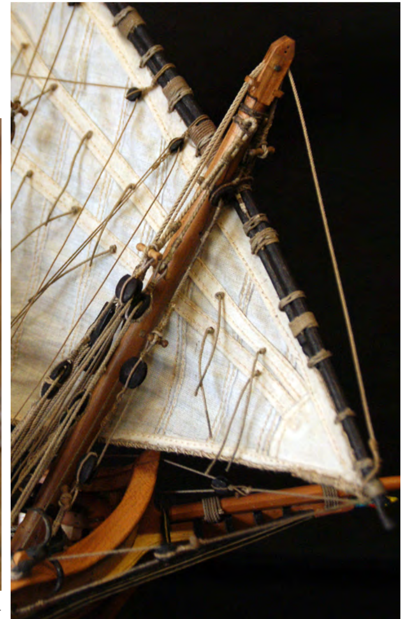
of a tackle whose other single block is seized to an eyebolt at the foot of the mast. The fall of the tackle belays to the bulwark.
