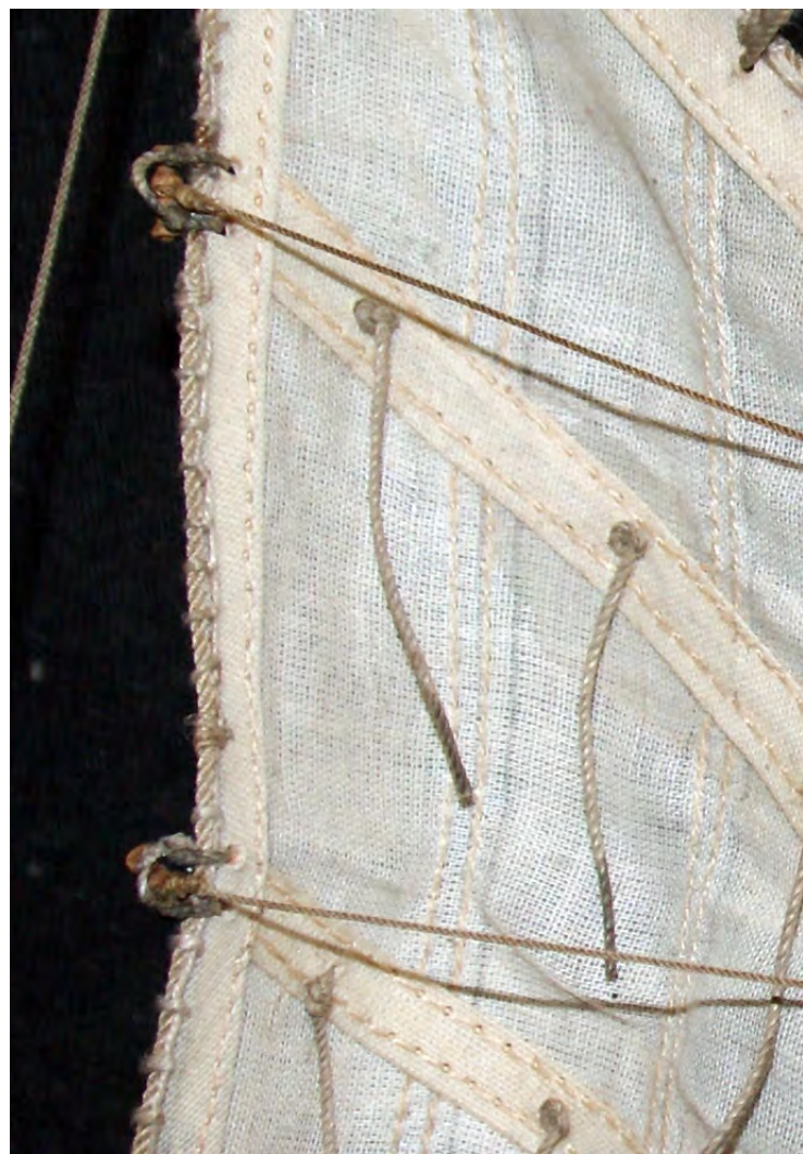
Photo n°. 268: Detail of the cringle on the leechrope for the top brail (131).
