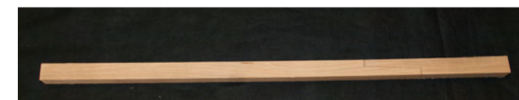
Photo n°. 40: Construction with a lathe is best and more precise and simplifies the work. Start with the circular portion of the mast, knowing that the section is not cylindrical but cone-shaped, getting smaller toward the head of the mast.
