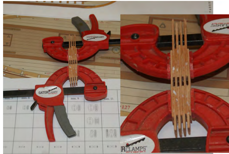
Photo n°. 180: The construction of the large and smaller halliard blocks (tailles in Mediterranean parlance), is similar. I prepare wood sticks that I glue together, leaving space for the sheaves in mortices. Originally these blocks were made of elm wood.
