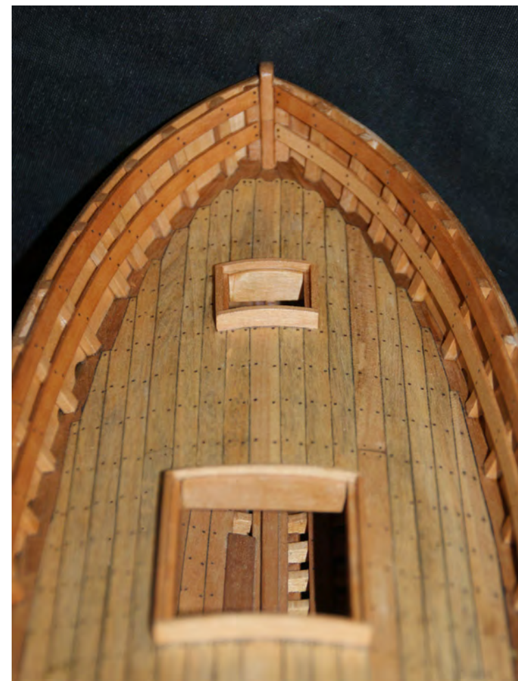
Photo n°. 102: Overhead view of the stern - bulwark planking (38) and ceiling (39). Bulwark planking strakes dimensions: 1.5 x 5 mm Ceiling strake dimensions: 1.5 x 5 mm
