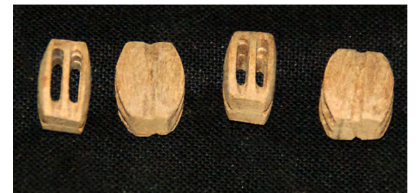
Photo n°. 205: Completed double blocks, ready for the sheaves.
