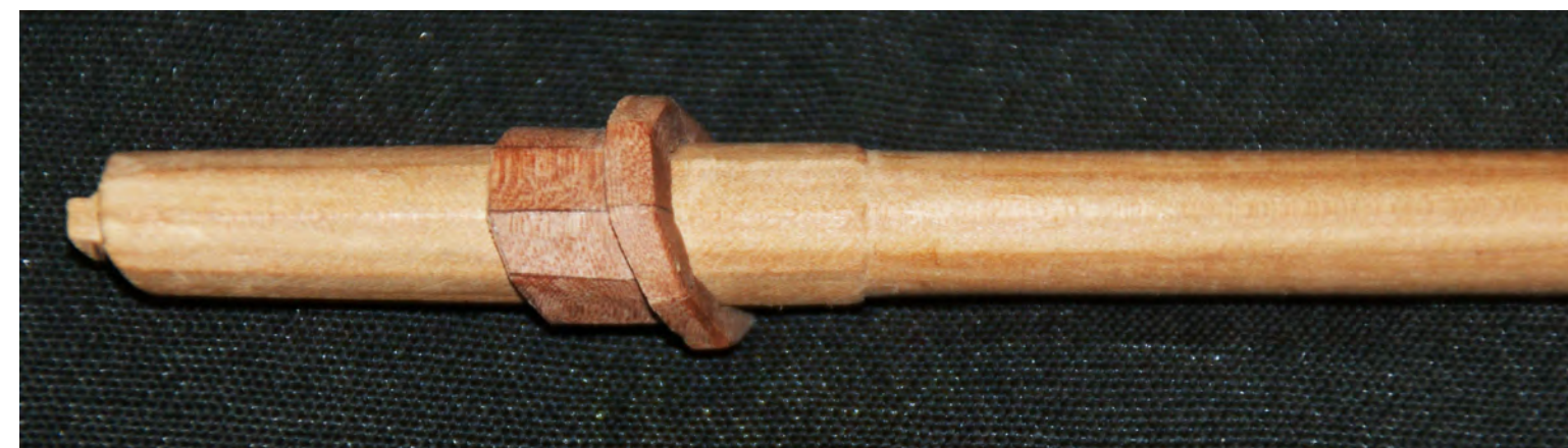
Photo n° 57: Foot of the mast with the wedges assembly in place. Note the strong angle obtained when the wedges were cut on a slant.
