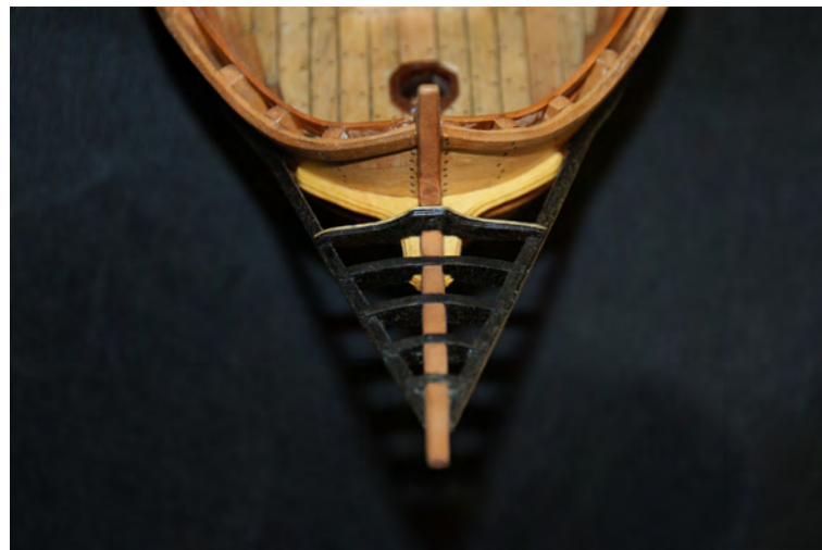
Photo n°. 100: Overhead view of the head with the five small beams in place.
