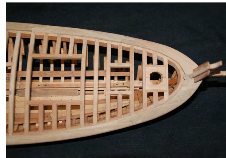
Photo n°. 38: We now proceed with the construction of the mast partners and the wedges that are necessary to maintain the masts in place. This photo shows the foremast partners and wedges. The thickness of the wedges (31) and (32) is 4 mm. Before completing the eight-sided hole, it is recommended to complete the masts and wedges in order to insure the correct rake of the wedges. Foreward rake of the foremast: 19.
