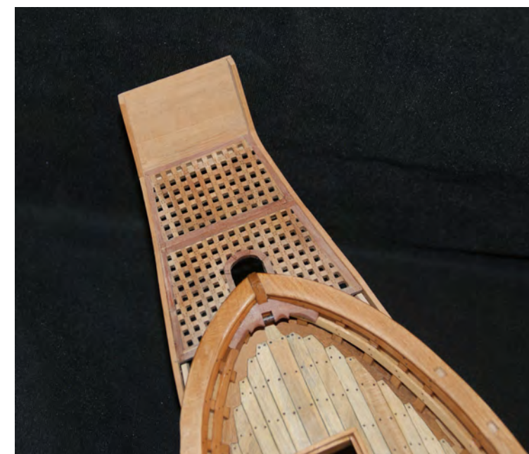
Photo n°. 120: Construction of the wings, inside view: the gratings and stern board have been installed.
