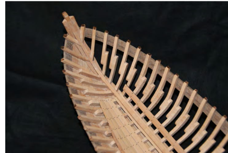
Photo n°. 31: The frames at the stem, footwaling and planking.
