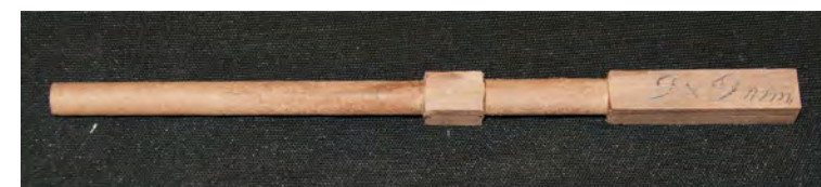
Photo n° 58: To start with, the piece is shaped on the lathe. Its length is taken from the drawing. You may retain the dimensions from my plates and follow drawings n° 10 and 11, or you may chose a drawing of your own.
