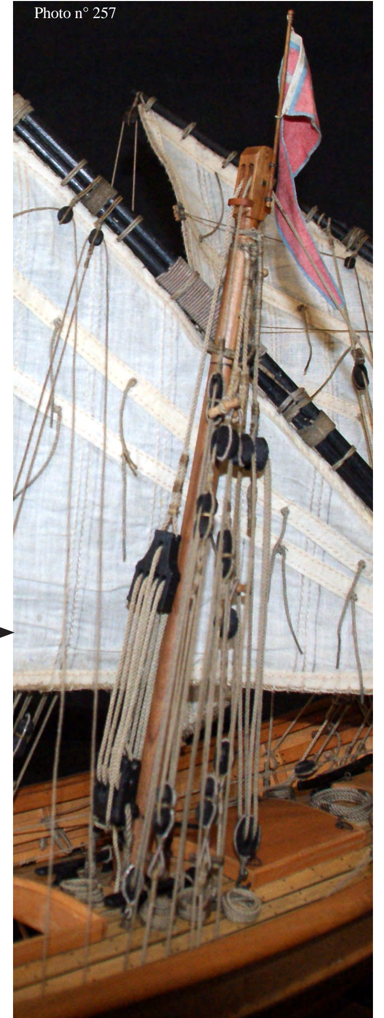
Drawing 43: The lift of the lower half of the yard and its tackle - rigging detail.
