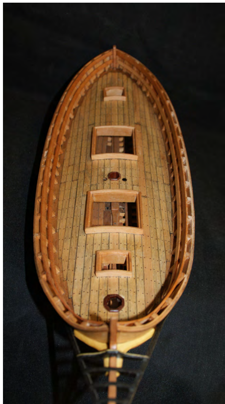
Photo n°. 101: Overhead view of the head and deck. The top rail will be installed later.
