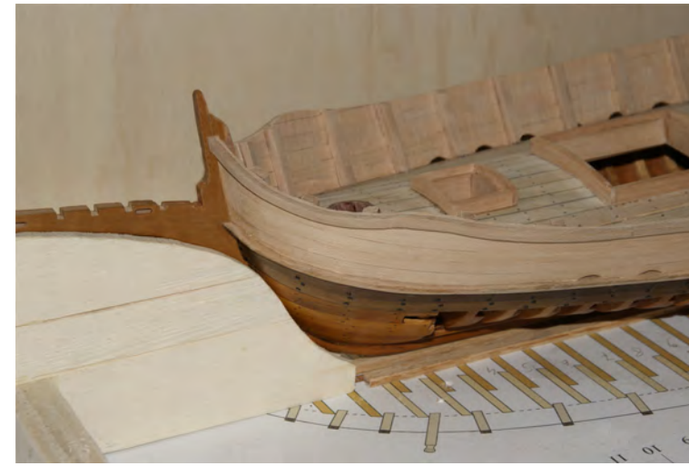
Photo n°. 83: Detail view of the head with the completed planksheer and planked bulwarks. Note the evolution in shape of the bulwark strakes.
