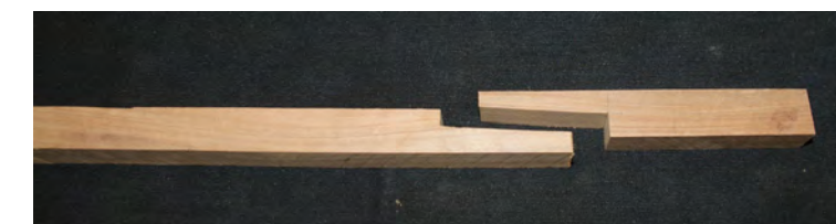
Photo n°. 39: We proceed with the construction of the mast after having joined and glued the two pieces.
