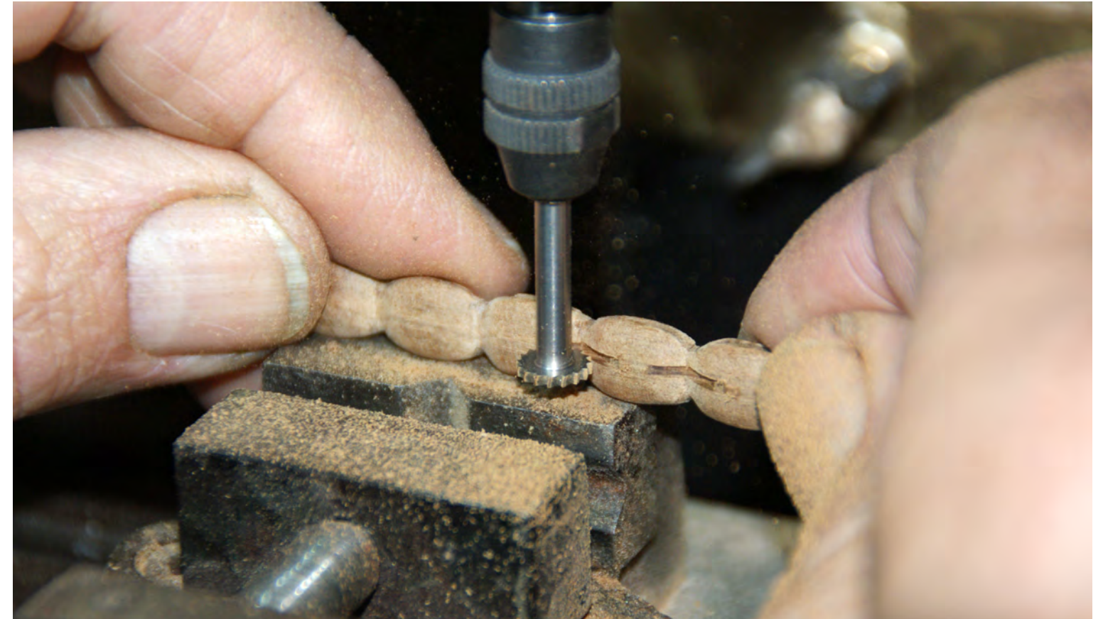
Photo n°. 203: Last step: milling bit n°. 4 is used to cut the recesses for the strops.
