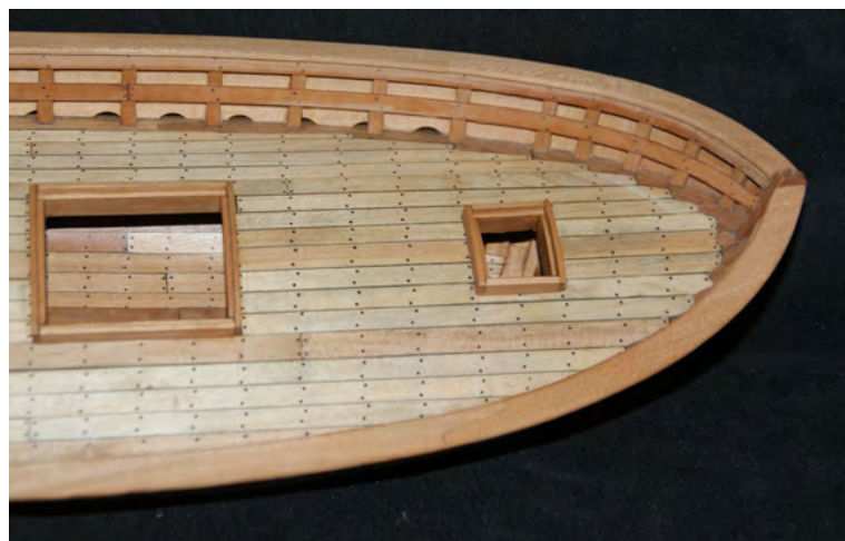
Photo n°. 109: Detail of the stern: top rail, sheer rail, bulwark rail, main and small stern hatches.
