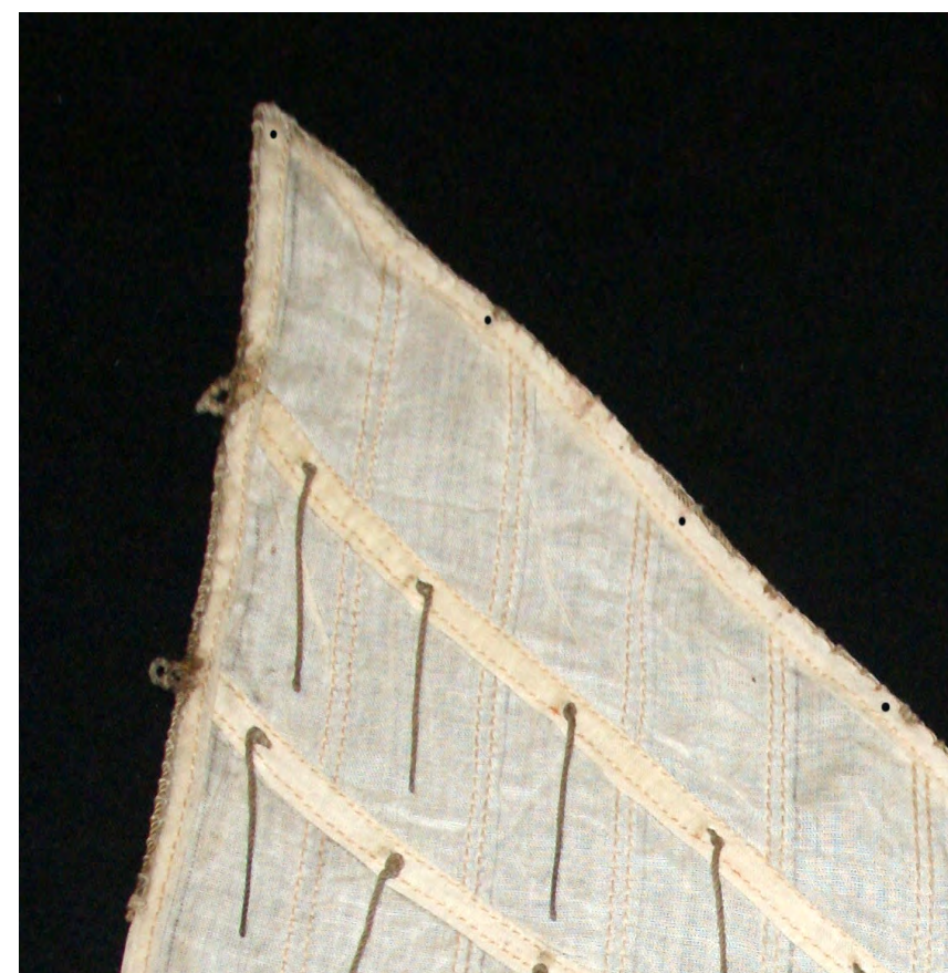
Photo n°. 217: The top angle (penne angle) of the foresail with two cringles and the reef bands and gaskets (matafions).
