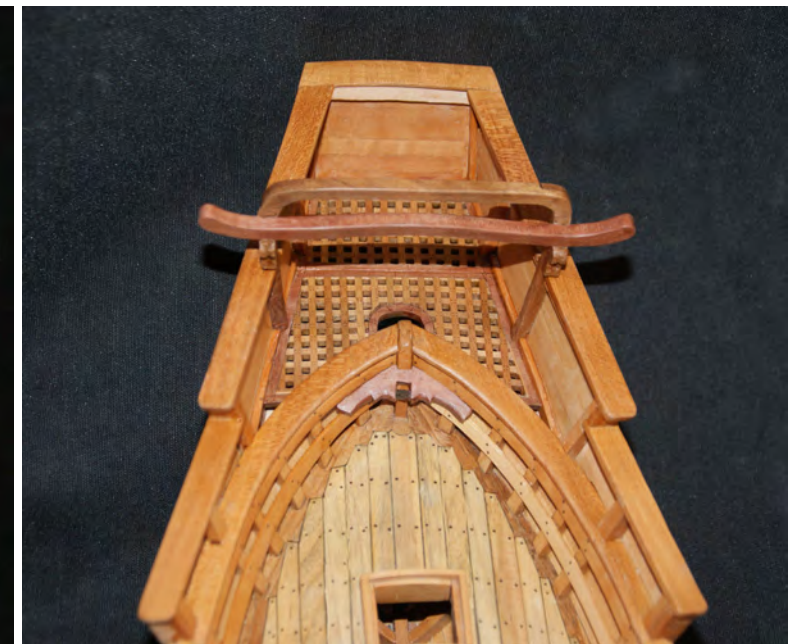
Photo n°. 133: The almost-completed cadrega. Installation of the arch the wings cross-beam.
