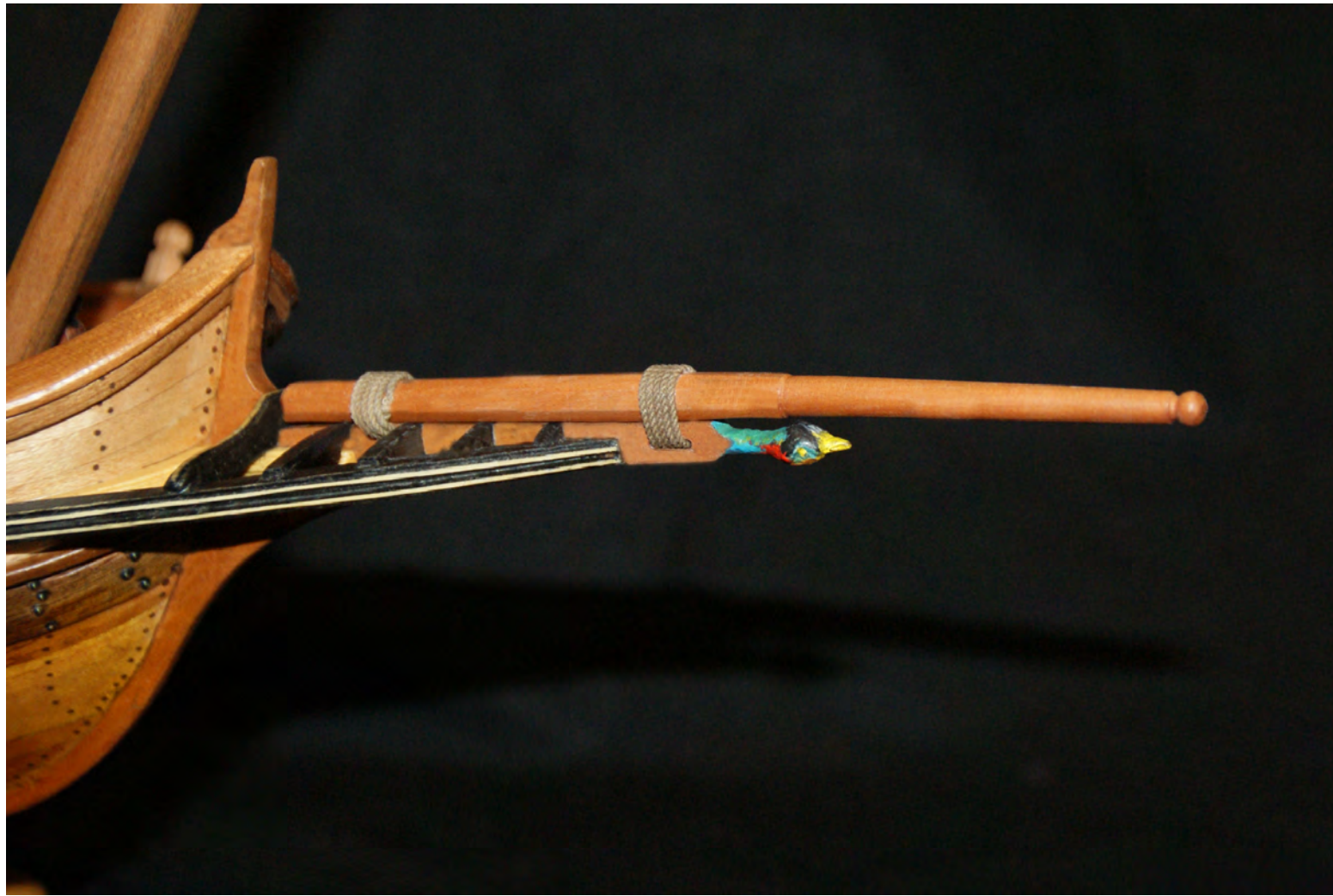
Photo n°. 172: The berthelot in lace on top of the beak. The gammoning (1.00 mm line) holds it to the beak.
