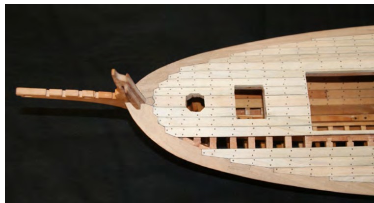
Photo n°. 68: Deck planking at the stem - foremast partners and small,hatch.
