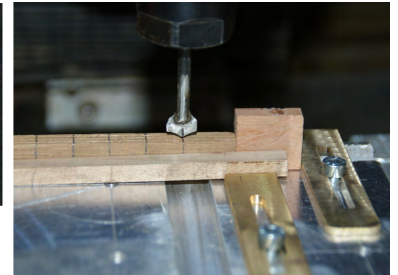
Photo n°. 198: Step two: using my tool n°. 1. I use it as a milling tool to shape the upper part of the shell.
