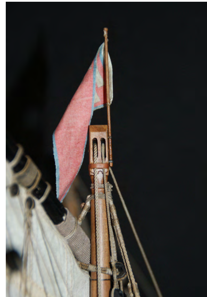
Photo n°. 252: Detail of the main masthead with its two sheaves, the halliard tie and the lift.
