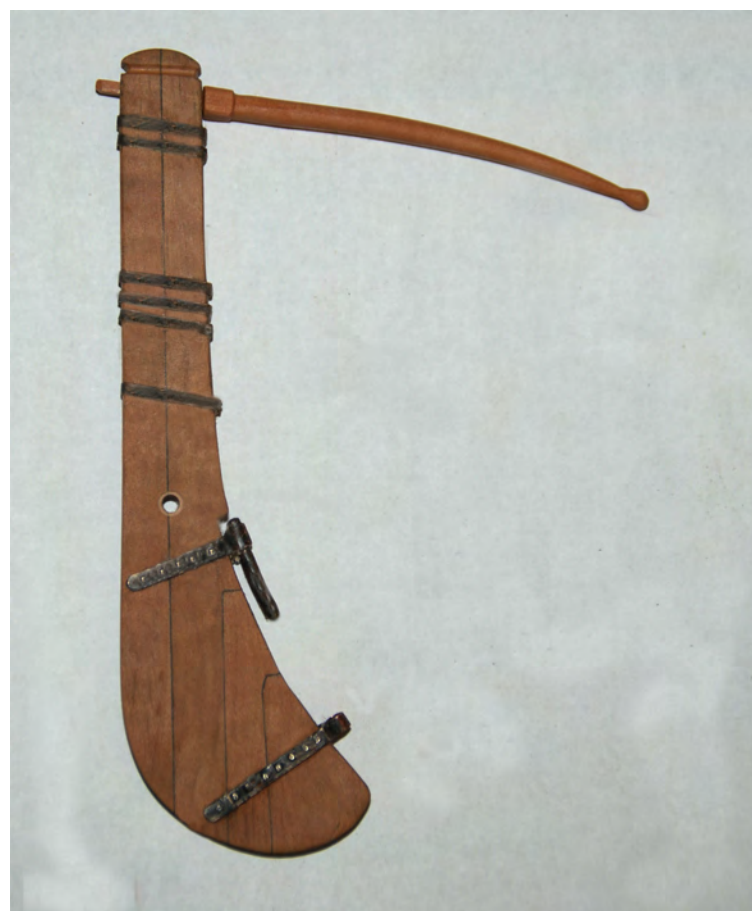
Photo n°. 118: The completed rudder with tiller in place. A hole for the rudder preventer rope next to a pintel and below, a gudgeon.
