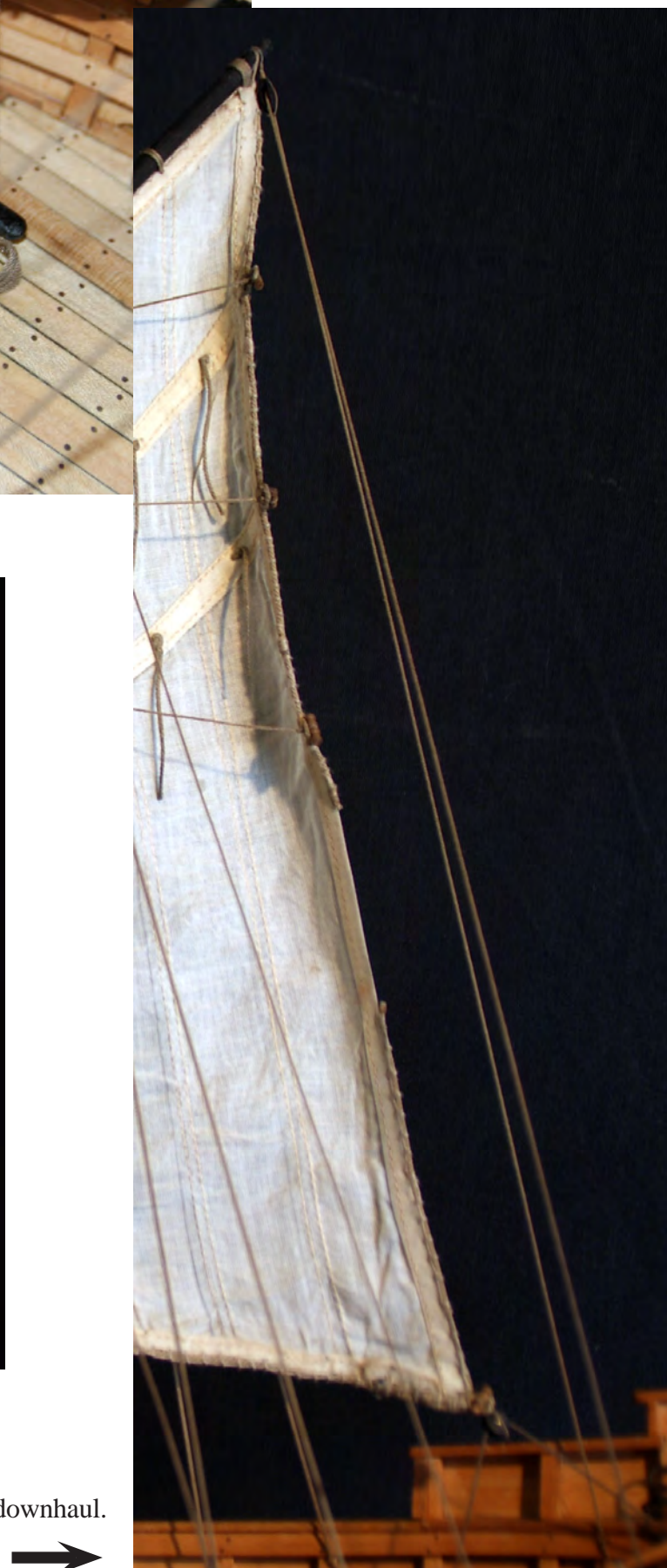
Photo n°. 266a: Detailed view of the block stoppped to the tip of the main yard.
