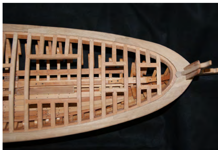
Photo n°. 37: Waterways - 12 x 3 mm - outboard thickness 3.5 mm.
