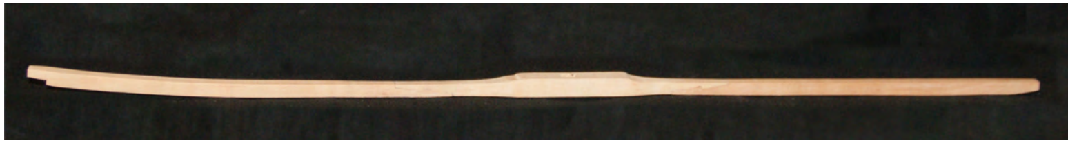
Photo n°. 26: Side view of the three pieces of the keelson after assembly.
