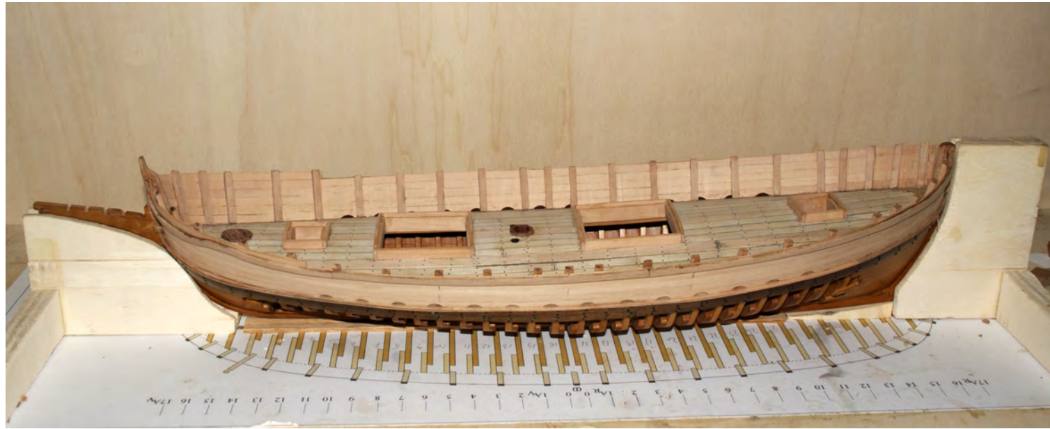
Photo n°. 80: Side view of the hull with the gunwale completed but needing to be finished-up.
