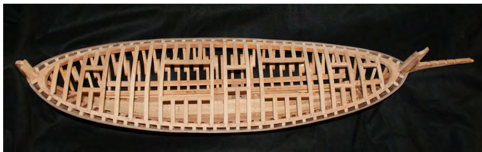
Photo n°. 36: Overall view of the deck structure: breast-hook and stern-hook, deck clamps, light deck beams (28) and half light deck-beams (28) are all in place. Starting from the stem, the first opening ready to receive the foremast partners (29), the second opening is for the small hatch (36) and the sixth one is for another small hatch (36).
