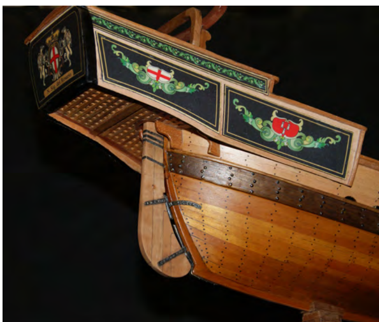
Photo n°. 157: Underside view of the stern decorations, the stern-board, the rudder ironwork, the gratings and the rudder.
