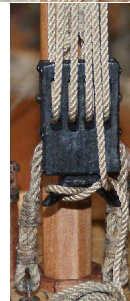
Photo n°. 230b: Detailed view of the upper large block. The fall of the tie reeves through the top of the large block, and is seized back to itself with three bindings.
