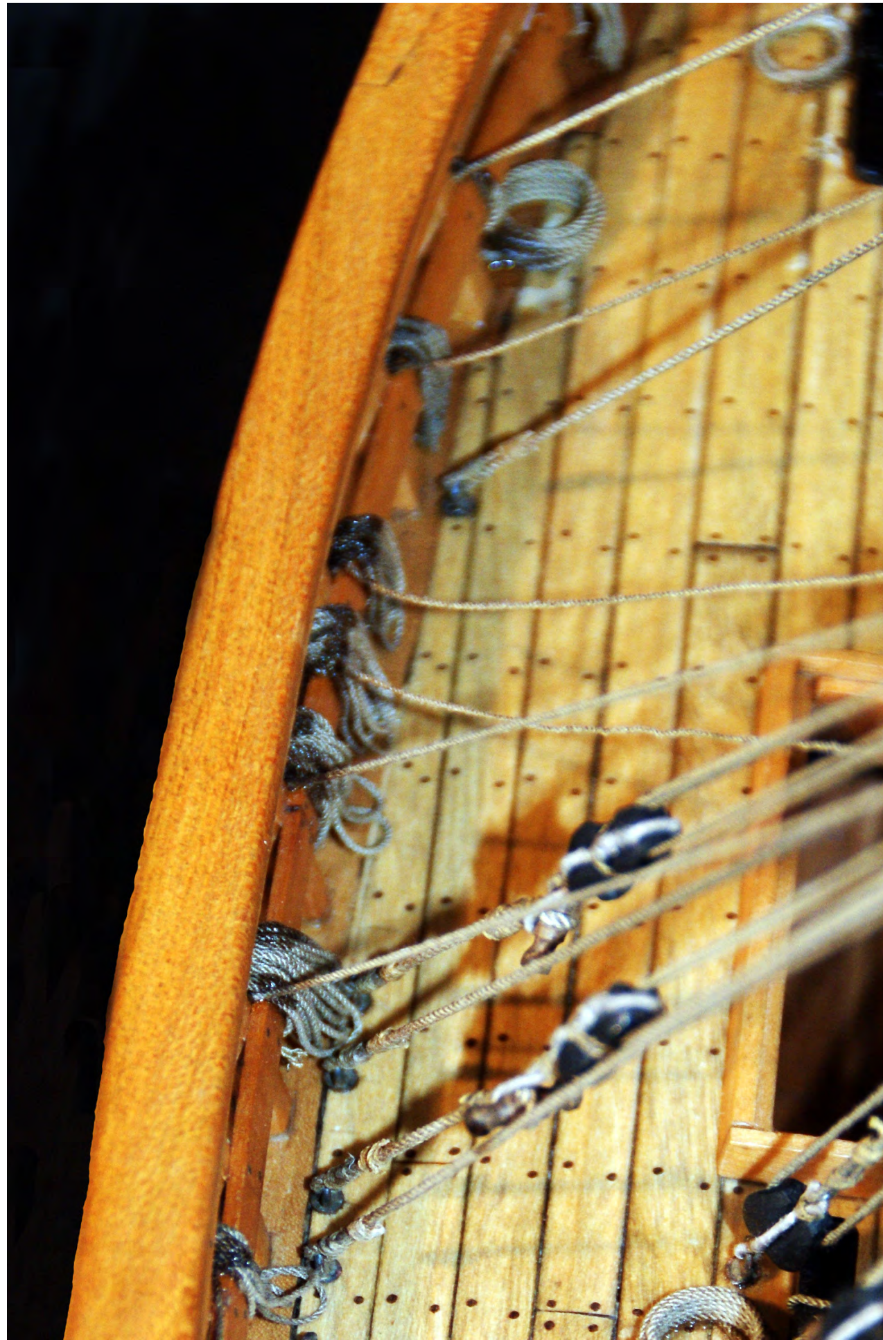
Photo n°. 269: Detail of the brails (131), (132), (133) belaying points on the bulwark strake(39).
