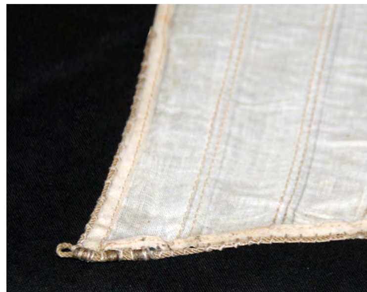
Photo n°. 215: Detail of the boltrope sewn to the sail edge and the thimble at the clew.
