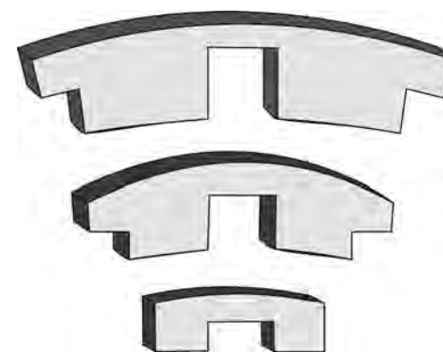
Drawing n°. 14: Small knees 3, 4, and 5. As for small knee n°. 2, The ends are dovetailed to the main rails and the middle notch fits on top of the beak.
