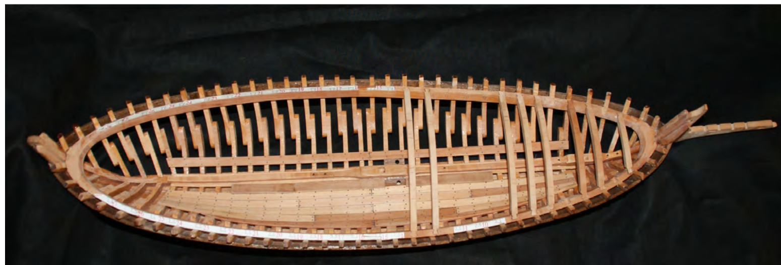
Photo n°. 35: The breast-hook and stern-hook, the deck clamp (27) and some deck beams all in place.
