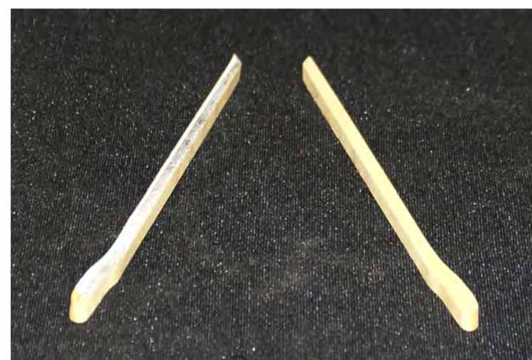
Photo n°. 94: The two parts of the main rail have been separated and ready to cut the bead.
