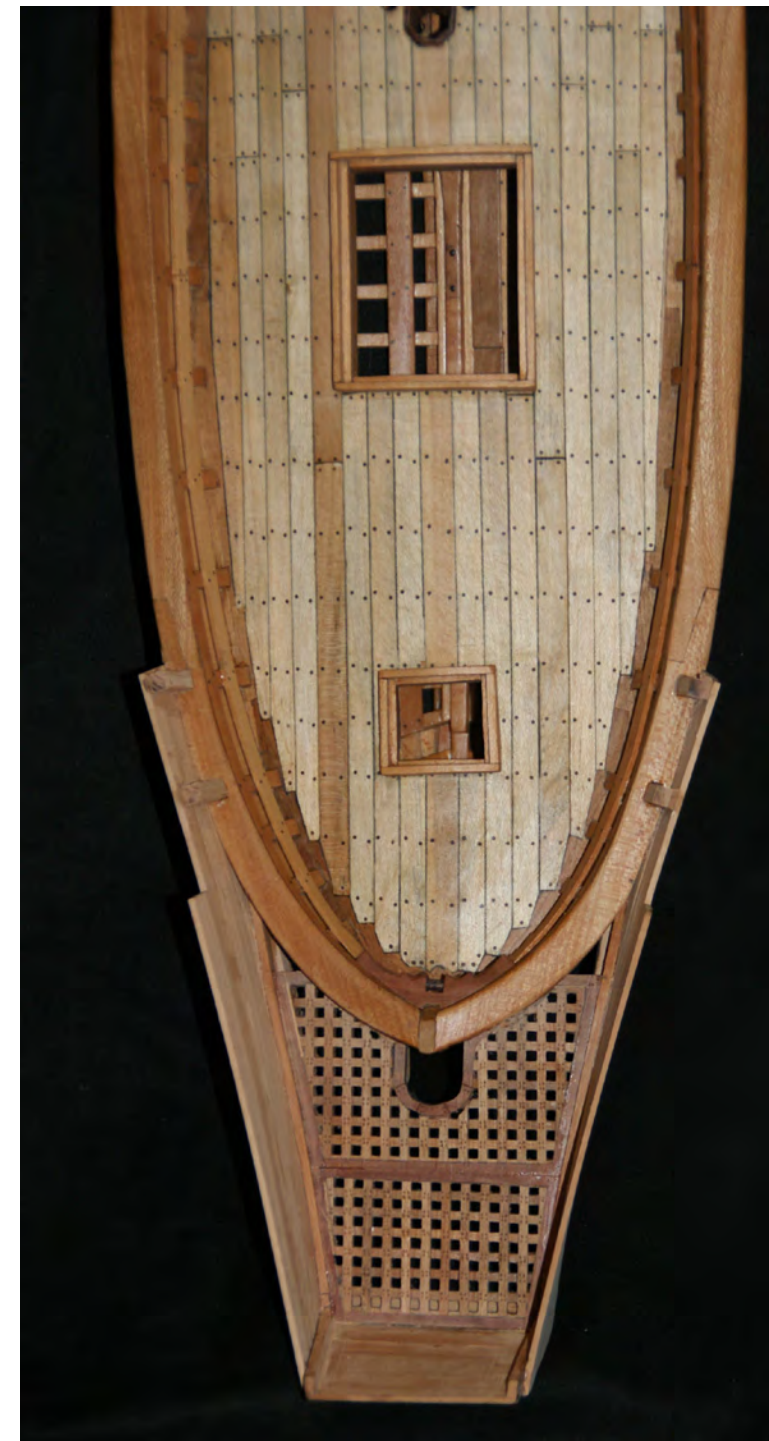
Photo n°. 131: Overhead view of the stern area, detail of the helm-port for the rudder post.
