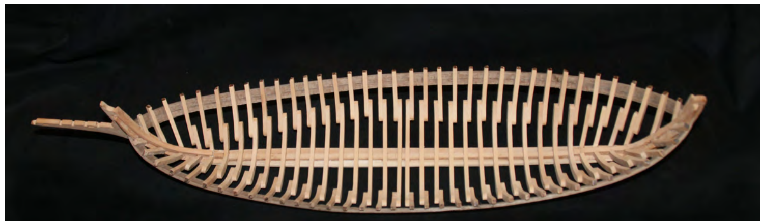
Photo n°. 29: The outer wales (58) and the keelson are in place. The structure is now ready to receive the footwaling (24).
