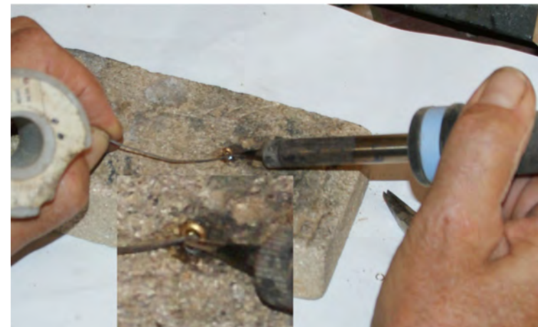
Photo n°. 178: Completion of the eyebolt. Slip a ring on the shaft, place the whole on a heat-proof pad, and solder with tin solder. The heat-proof pad is a Magnsia Solderin Block and may be purchased in the US: http://www.ottofrei.com .
