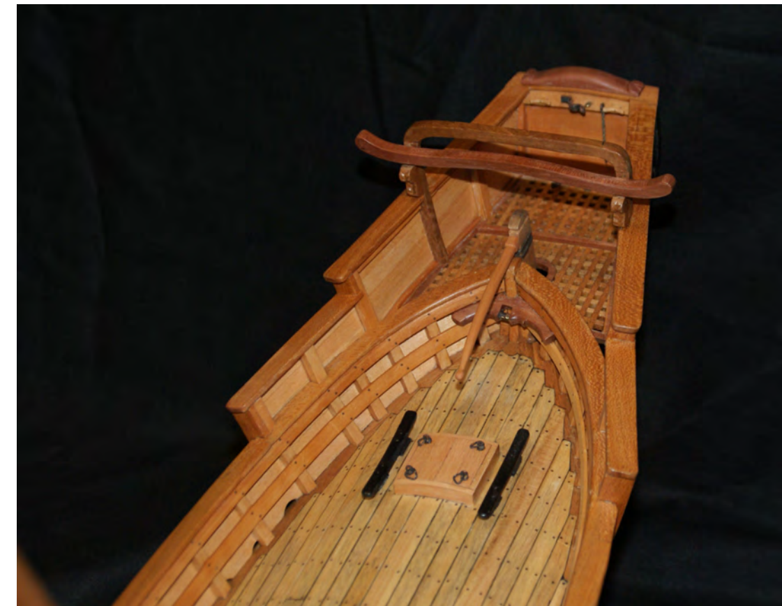
Photo n°. 150: The stern is complete! Note the structure of the wings, the tiller, the small stern hatch with its cover and cleats to the sides.
