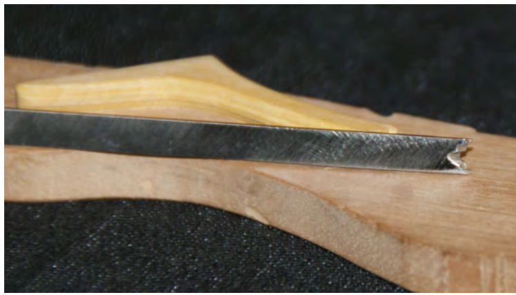
Photo n°. 89: The tool used to construct the parts - I use an old hacksaw blade that I file to the desired shape.
