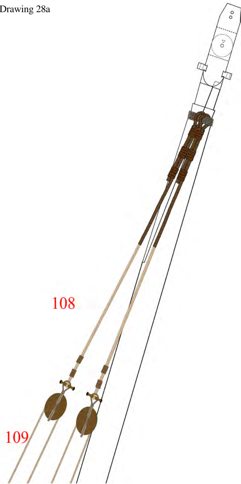
Drawing 28a: The standing end of the pendant is seized to the lower slot in the mast, n°. 108. Drawing 28b: The standing ends of the switching shroud. Drawing 28c: Lower standing end and bowser of the switching shroud (110 and 111).
