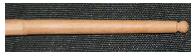
Photo n°. 170: Detail of the berthelot: the truncated-cone section and the ball at the tip. The curvature can hardly be seen on the picture.
