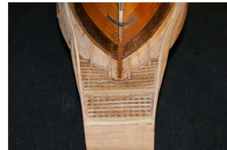
Photo n°. 122: Overhead view of the stern. One may visualize the small beams that support the gratings, the support timbers, as well as a cross-beam underneath.
