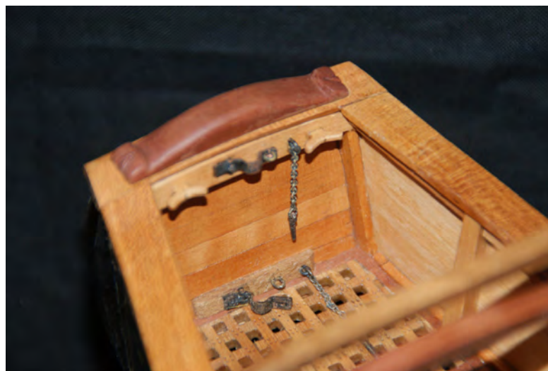
Photo n°. 136: Detail of the inside face of the stern board, ironwork for the installation of the flagstaff. Two hinged collars (73) locked by pins hanging from an eyebolt with a small chain, two small cleats for the flagstaff halliard.
