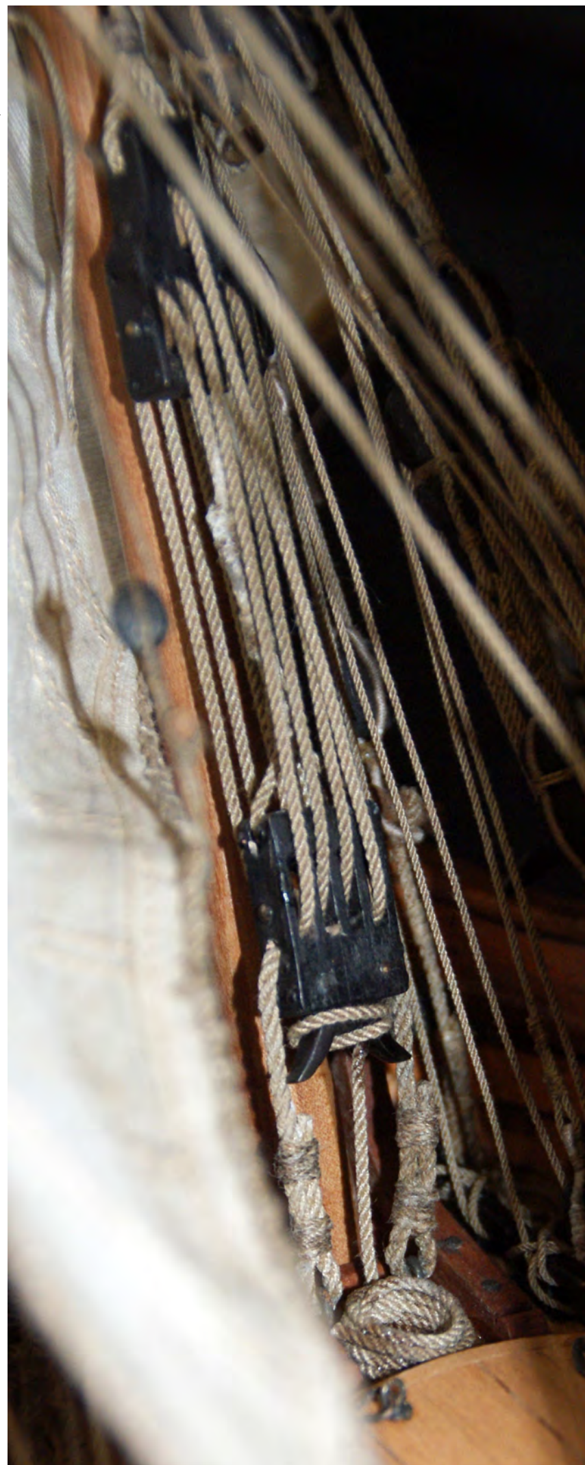
Photo n°. 229: Detailed view of the halliard tackle (103), 1.15 mm diam. - the two upper and lower large blocks.
