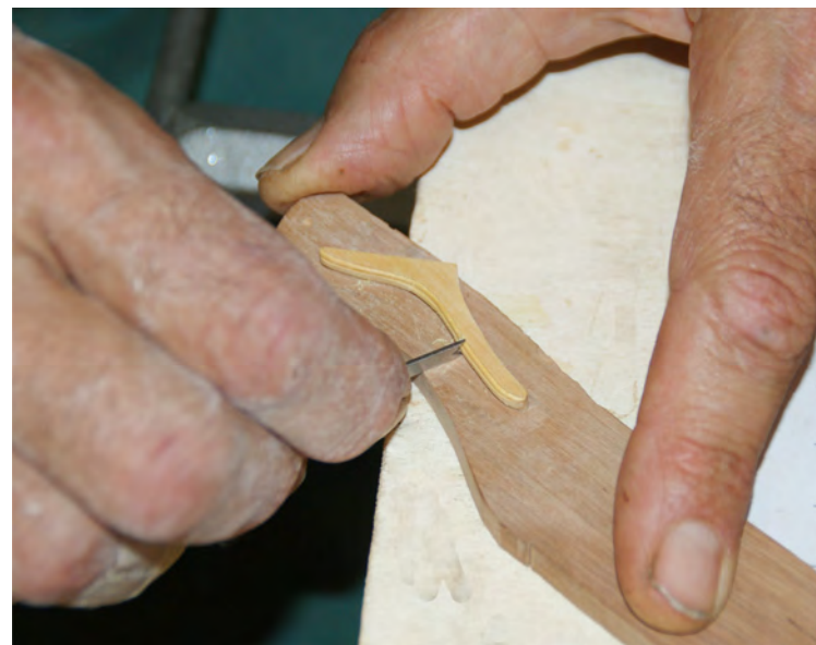
Photo n°. 90: To cut the molded bead in the best conditions, I glue the part to a smooth piece of board to insure that the tool will slide smoothly. Once the cutting work is complete, I remove the part using a solvent (acetone will dissolve any glue, even cyano).
