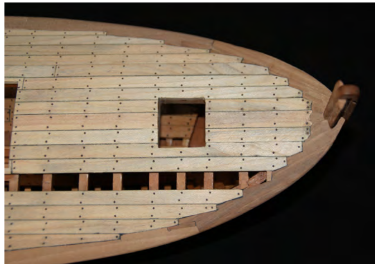
Photo n°. 70: Deck planking at the stern and the small hatch. The deck nails are 0.6 mm in diameter.
