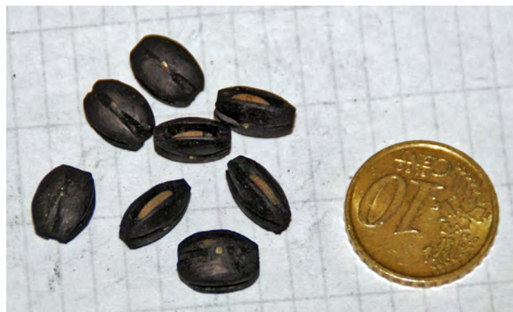
Photo n°. 206: Completed single blocks.
