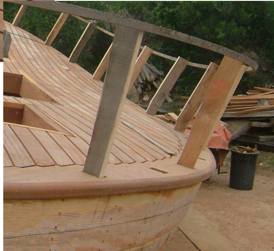
Photo n°. 77a: Photo of a real ship. Note how the holes for the risers are made.
