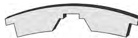
Drawing n°. 13: Small beam n°. 2. The middle, rectangular notch fits on the beak. It is connected at its ends to the main rails with dovetails.
