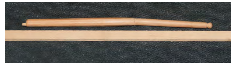
Photo n°. 168: The comparison with a straight stick shows the amount of curvature to be given the berthelot.
