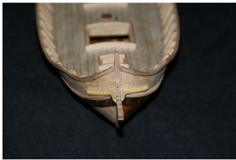
Photo n°. 92: A front view of the small knees glued to the hull - we can start the head timber and main rails. Head timber dimensions: 3 x 2 mm.
