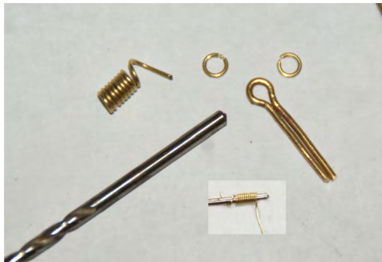
Photo n°. 177: An eyebolt, a spiral and two rings, with the drill bit used to make the spiral. We now go on to finishing the eyebolt.
