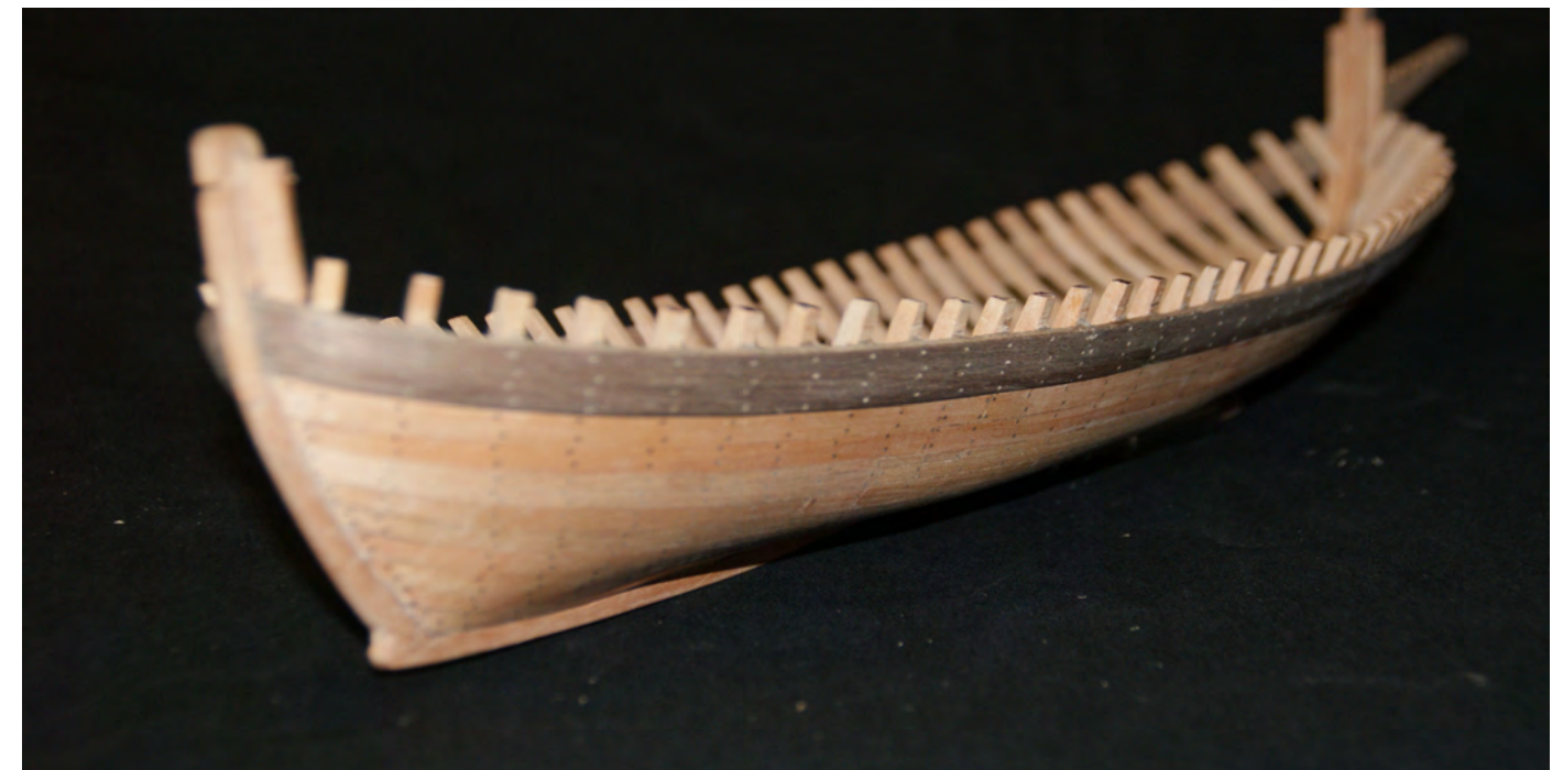
Photo n°. 32: The completed planking (64): 1.5 x 5 mm Nails for the planking: 0.6 mm
