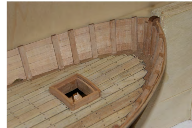
Photo n°. 84: A view of the inside of the completed gunwale at the stern.
