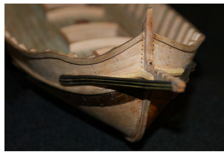
Photo n°. 95: The main rails are in place - The five small beams may now be prepared.
