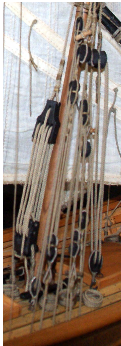
Photo n°. 259: The lift in the foreground (138); At the top, the fiddle block and at the bottom, the single block.
