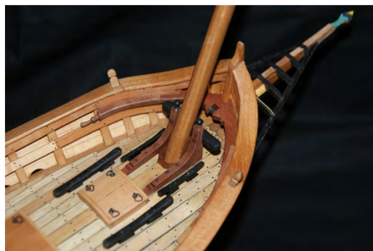
Photo n°. 155: As before: Detail of the riding bitts and the breasthook.
