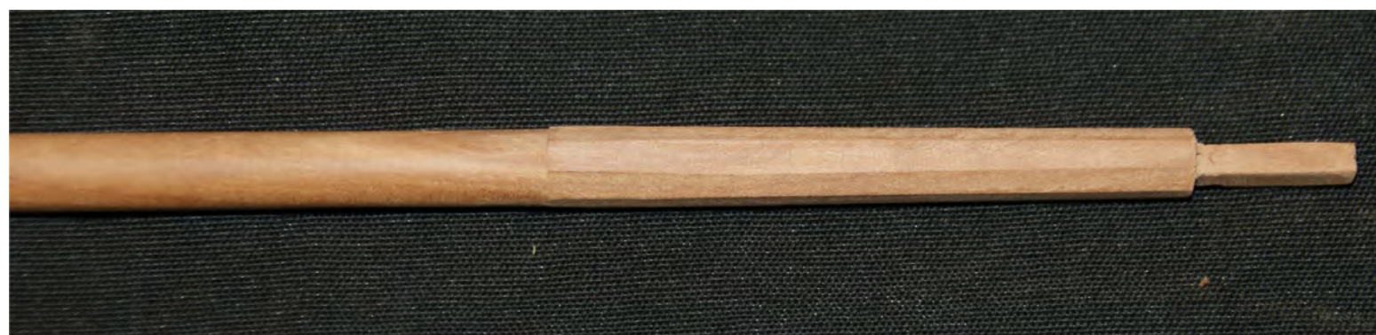
Photo n°. 44: The section of the masts that is below-deck is eight-sided and ends in a square tenon that engages in the mast step on the keelson.
