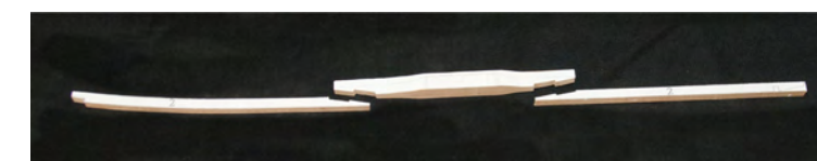
Photo n°. 23: We can see a side view of the three pieces making up the keelson. In the center is the piece that takes the mainmast step.
