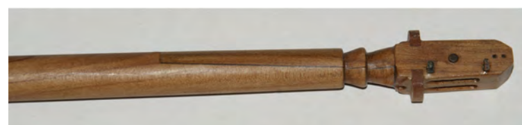
Photo n° 51: The completed masthead with « calcet ». Two eyebolts for the mast-head pole have been added.
