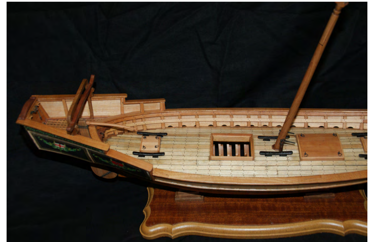
Photo n°. 151: Starboard port. The structure of the wings, the tiller, the small stern hatch and its cover, the cleats on the sides, the open after main hatch, the mainmast with the pumps and cleats to the sides, the fore main hatch and its cover.
