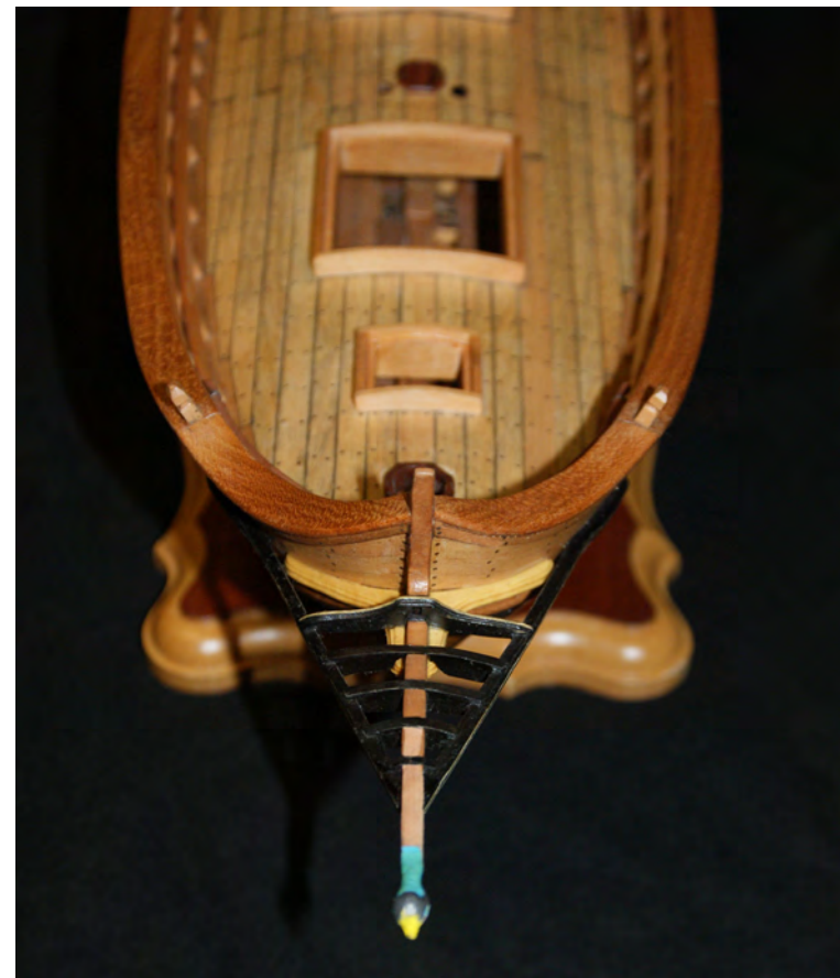
Photo n°. 146: Construction of the stem. At the tip of the beak is a carved bird.
