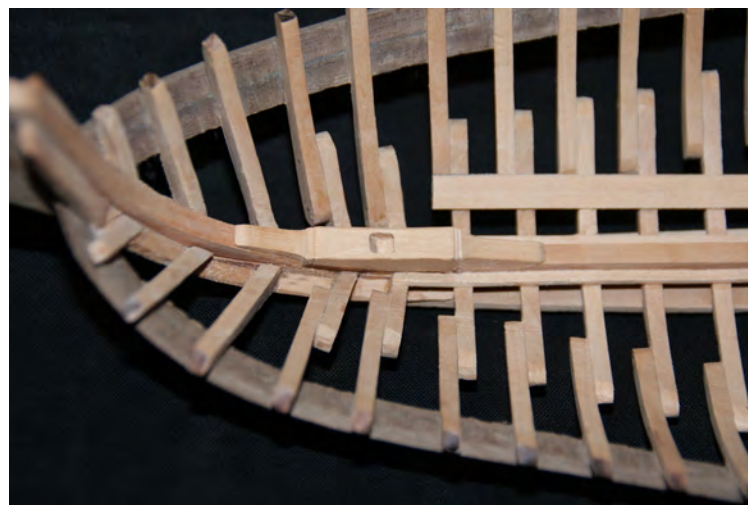
Photo n°. 28: The fore section of the keelson that the foremast (22) step is assembled on - note that it is wider than the keelson at that point.
