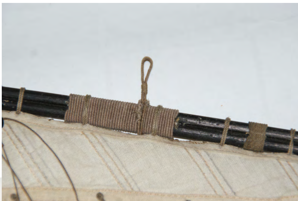
Photo n°. 220: The sling « polome » (G146 or G 147) - a double rope that wraps around the yard at about 1/3 its length and is used to tie it to a tackle to raise it (see yard halliard). It is wrapped twice around the yard and makes a slip-knot.
