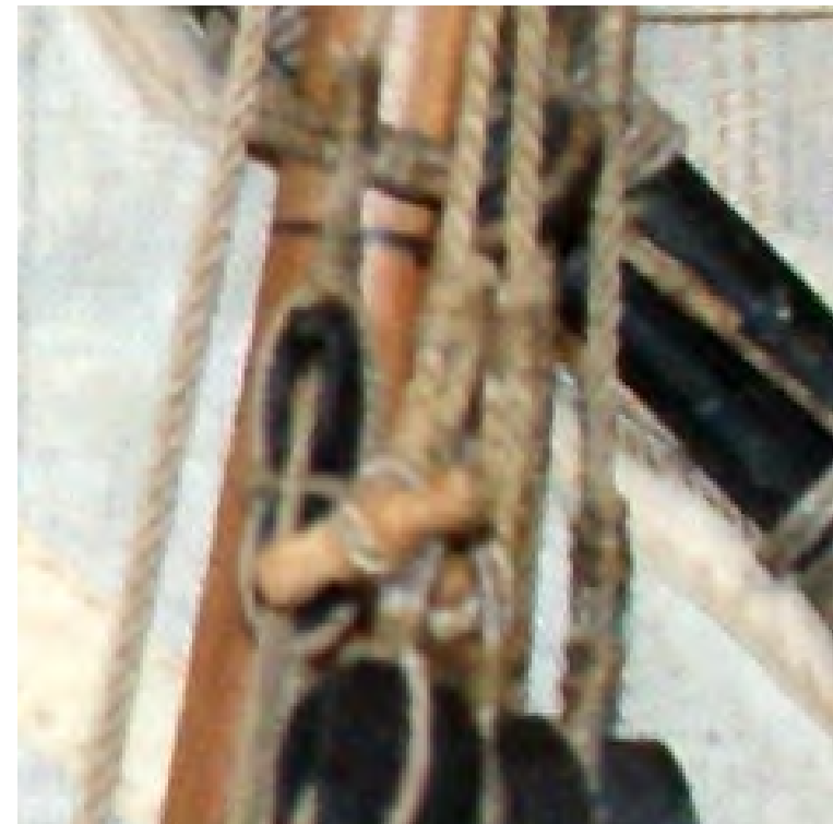
Photo n°. 259a: In the foreground, the lift of the lower half of the yard and at the top, the fiddle block.
