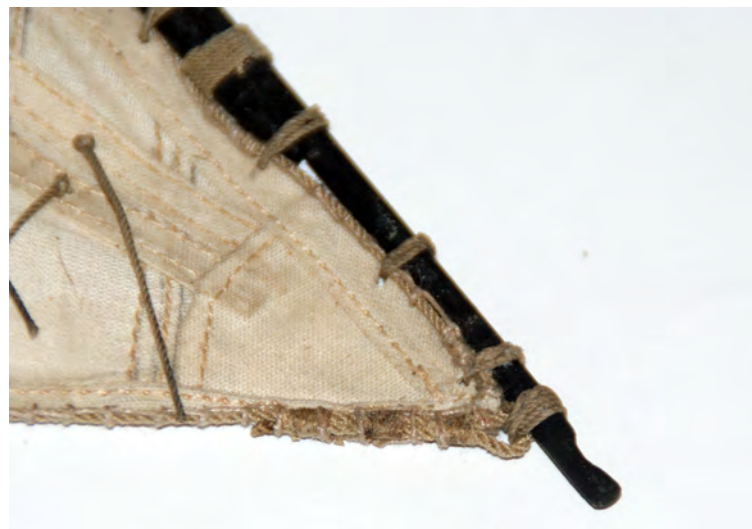
Photo n°. 219: Binding of the sail on the yard quarter at the brace point.
