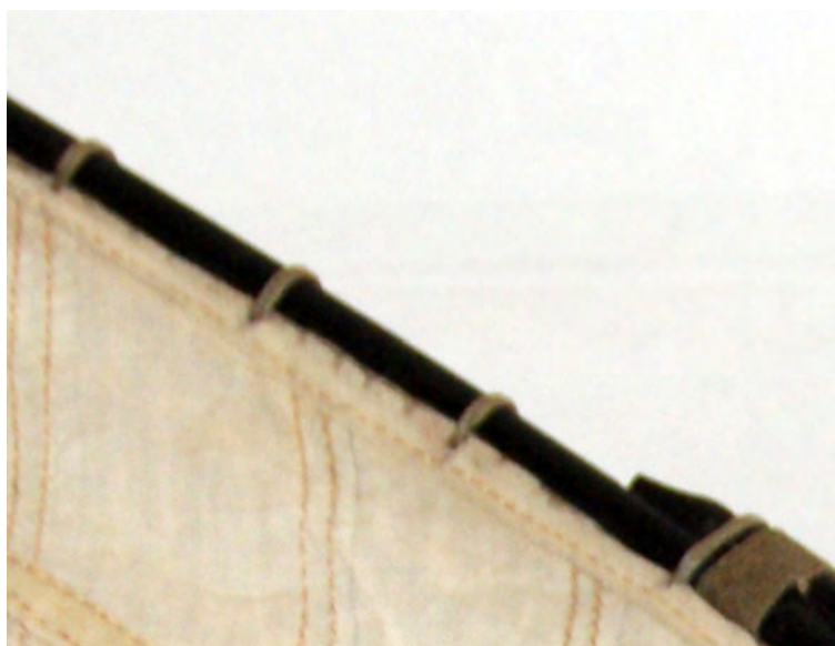
Photo n°. 218: The sail is bent to the yard with simple bindings.
