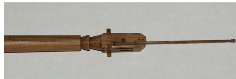
Photo n° 53: The « calcet » masthead with the masthead pole inserted in the eyebolts.
