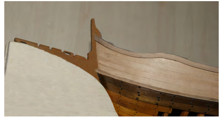
Photo n°. 86: Detail of the head with the completed gunwale and top rail. Note the increased curvature of the top rail.
