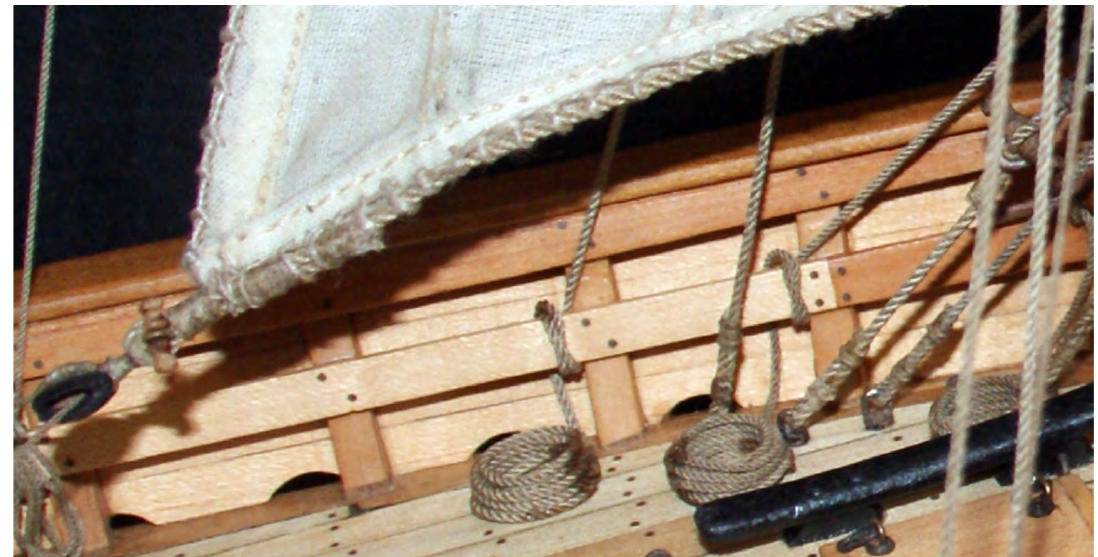
Photo n°. 241: Detail view of the foresail sheet. In this case, it belays on the large cleat on deck, reeves through a single block and returns to a strake on the bulwark. The
