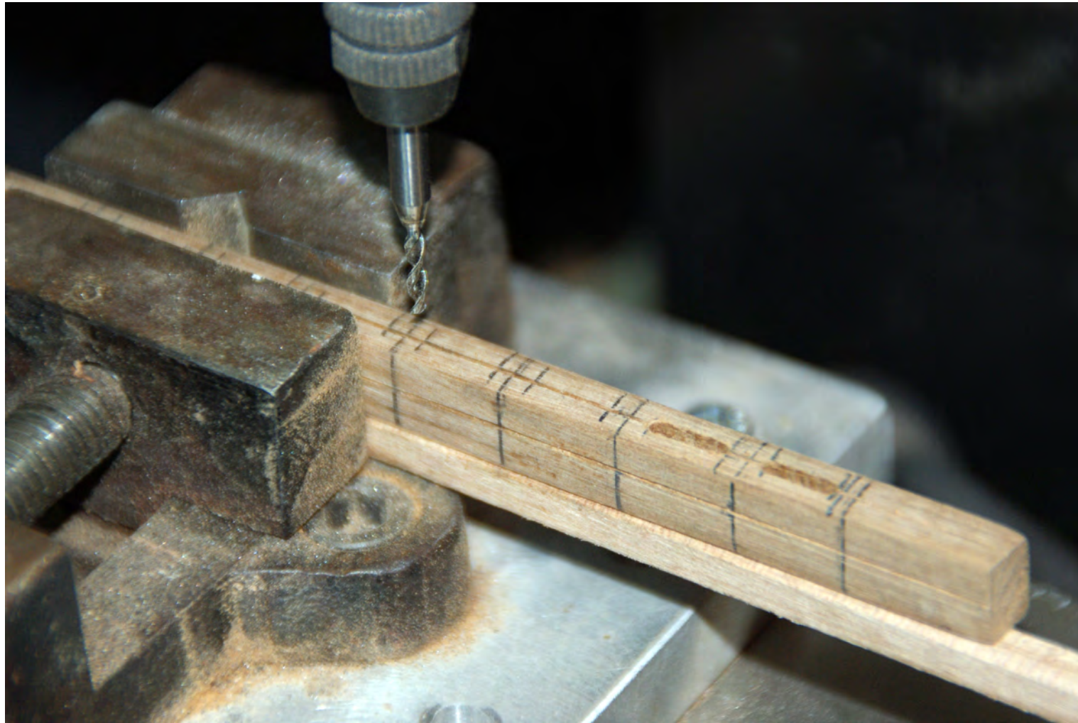
Photo n°. 200: Step four: Drilling out the body of the block using tool n°. 3, a milling bit.
