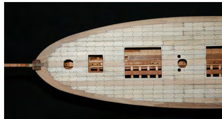
Photo n°. 71: Completed deck planking forward.
