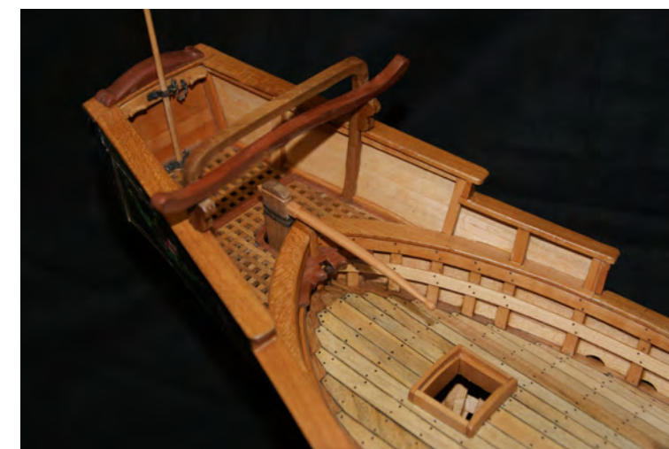
Photo n°. 140: Completed structure of the stern. The top of the rudder juts through the helm-port and the tiller is in place.
