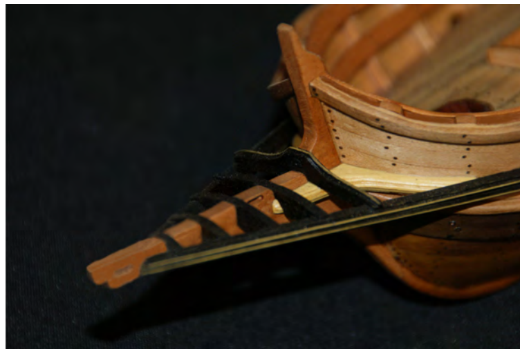
Photo n°. 99: Side view of the head: the small beams are in place.
