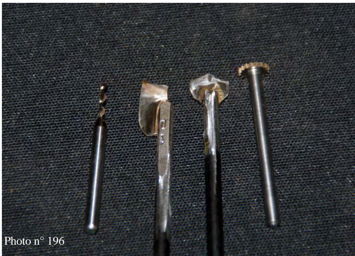
Photo n°. 196: In order to produce the blocks using my method, it is necessary to make some cutting tools. Two are needed for each block size. I will explain the use of these home-made tools in the following photos.
