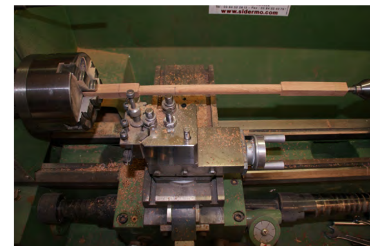
Photo n°. 41: Next, provide the two sections that will serve to hang the pendants of the switching shrouds.
