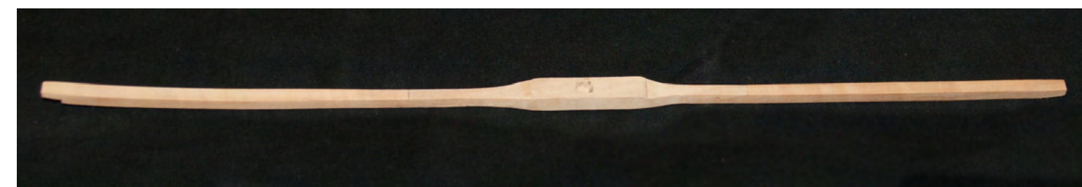
Photo n°. 25: Top view of the three pieces of the keelson after assembly.
