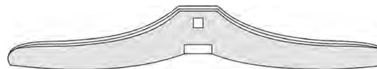
Drawing n°. 12: Small knee n°. 1. The square opening is for the bowsprit (bertelot) step; the rectangular notch fits into the beak.
