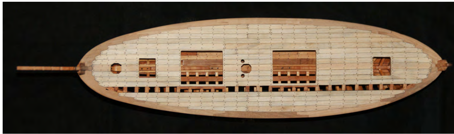
Photo n°. 67: The plank laying and nailing of the deck have been completed. One strake was not installed in order to show the coaming strakes - the planking strakes are thicker between the coaming strakes ( see drawing 11).
